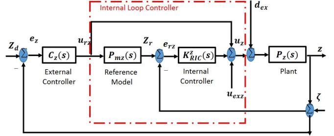
Fig. 4. RIC Disturbance Compensation Controller
