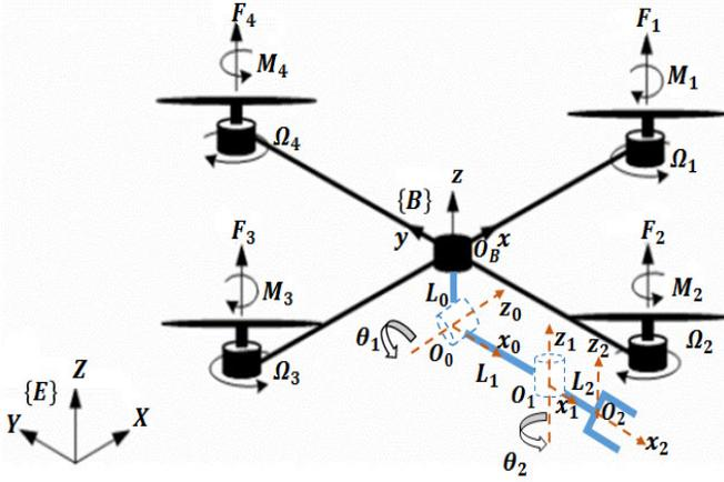
Fig. 2. Schematic of Quadrotor Manipulation System Frames
