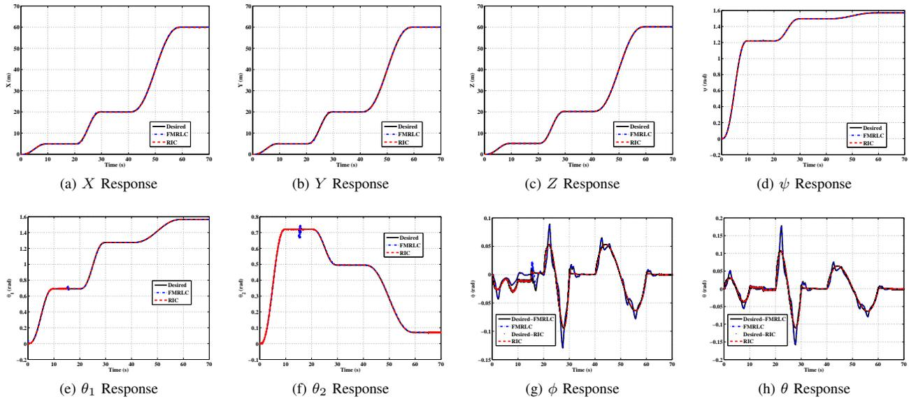
Fig. 5. The Actual Response of both RIC and FMRLC Techniques: a)  $X$ , b)  $Y$ , c)  $Z$ , d)  $\psi$ , e)  $\theta_1$ , f)  $\theta_2$ , g)  $\phi$ , and h)  $\theta$ .
