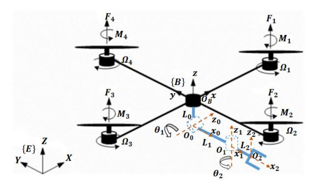
Figure 6: Schematic of Quadrotor Manipulation System Frames
