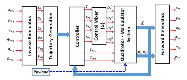
Figure 8: Block Diagram of the Control System
