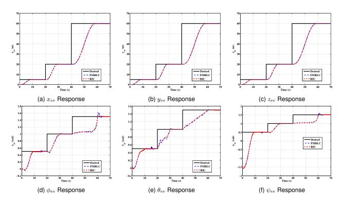
Figure 11: The Actual Response of both RIC and FMRLC Techniques for the End Effector Position and Orientation: a)  $x_{ee}$ , b)  $y_{ee}$ , c)  $z_{ee}$ , d)  $\phi_{ee}$ , e)  $\theta_{ee}$ , and f)  $\psi_{ee}$ .
