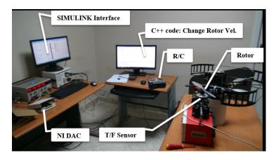
Figure 7: Experiment to estimate rotor coefficients
