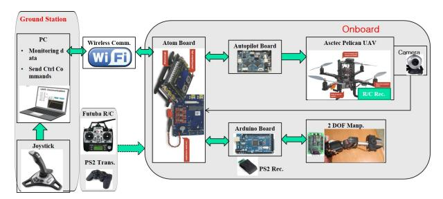
Figure 5: Aerial manipulation functional block diagram
