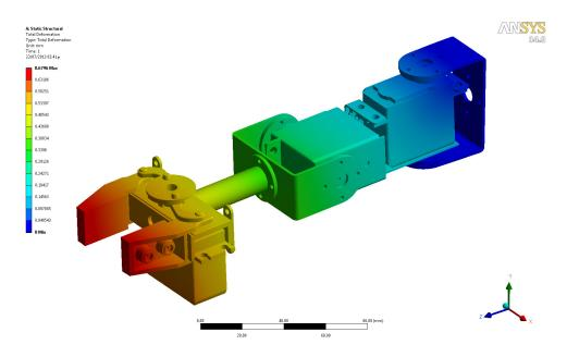
Figure 2: Manipulator's structure deflections using ANSYS
