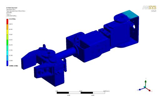
Figure 3: Manipulator's structure stress analysis using ANSYS
