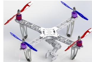
Fig. 2. 3D CAD model of the New Quadrotor Manipulation System
