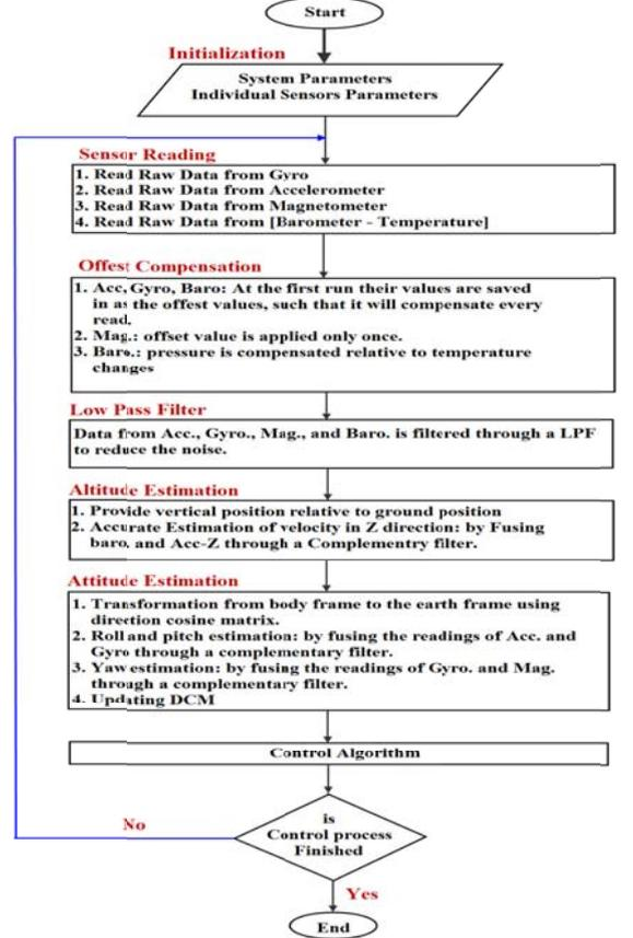
Figure 10. Flowchart for estimating attitude of quadrotor
