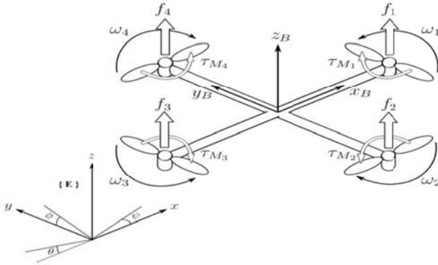
Figure 1. Schematic of Quadrotor System
