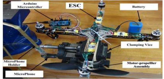
Figure 3. Test Rig for identifying Rotor Angular Speed
