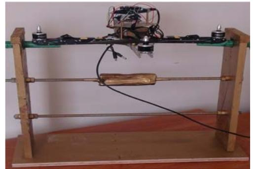
Figure 11. Roll, and pitch angle test rig
