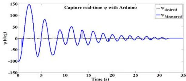
Figure 14. Experimental response of yaw controller
